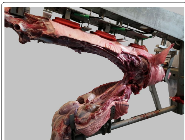
Fig. 2 The Meat Factory Cell's "Carcass Handling Unit". The limbs have been removed and the belly and ribs sawed approximately 12–15 cm from the spine. Then the truncus has been lifted up. Trachea, oesophagus with some soft tissue is available for the butcher
