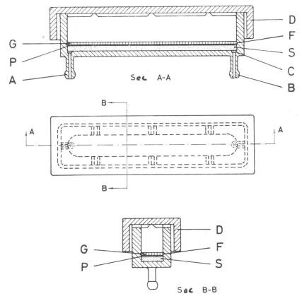
Figure 1. (A) Hose nipple. (B) Hose nipple. (C) Glass wool. (D) Lid. (F) Groove. (G) Agar. (P) Rice paper. (S) Sephadex.
