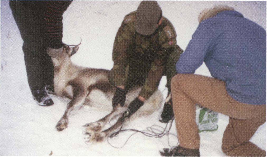
Figure 1. Measurement of radioactive caesium in live reindeer.
