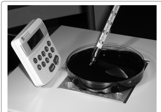
Fig. 1 Test apparatus. Gyrodactylus salaris individuals were attached on a rainbow trout fin that was placed in 65 ml of fish tank water. The temperature of the water was maintained (or raised by heating with a desk lamp in the second experiment on heat disinfection) by the heat block under the Petri dish and followed with the thermometer. The survival time of individual parasites was recorded with the stopwatch
