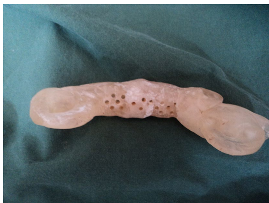
Fig. 1 A polymethyl methacrylate (PMMA) mouthpiece with holes specially constructed for the study, adjusted like a bit on a bridle. When the horse is chewing, saliva is collected in the reservoir. After removing the mouthpiece, the saliva can be emptied through a hole on the short side into an Ellerman polystyrene tube
