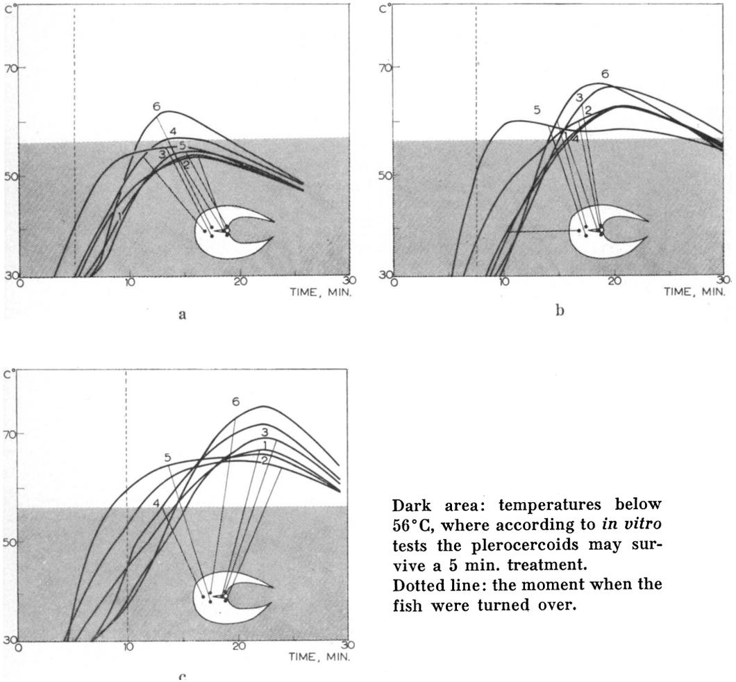
Dark area: temperatures below 56°C, where according to *in vitro* tests the plerocercoids may survive a 5 min. treatment.
