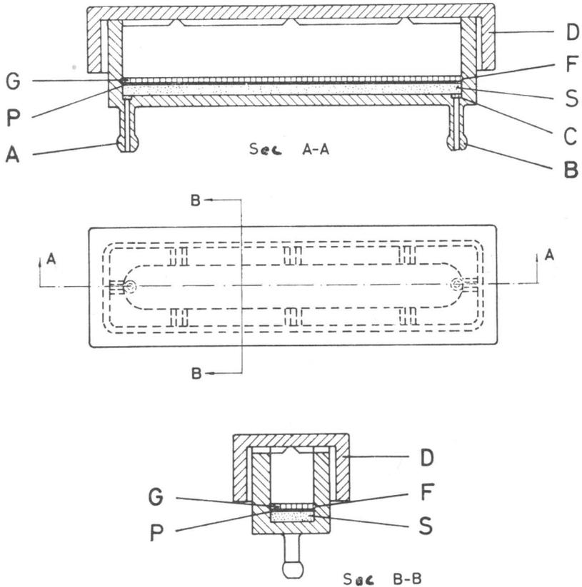
Figure 1. (A) Hose nipple. (B) Hose nipple. (C) Glass wool. (D) Lid. (F) Groove. (G) Agar. (P) Rice paper. (S) Sphadex.
