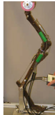
Fig. 4 Articulated replica of a canine pelvic limb fabricated using 3D printing. The patellar ligament is made using braided silk. The leg is held up within a frame and the hip joint is loaded. Quadriceps femoris and gastrocnemius muscle tones are simulated using metal wires. The knee angle is assessed using an electrogoniometer
