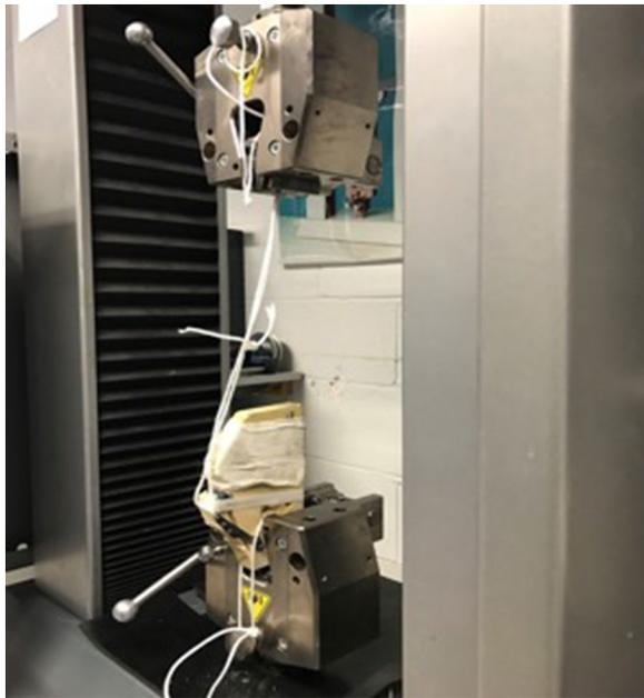
**Fig. 1** Image of the tensile testing machine used to measure tensile strength in the experimental samples
